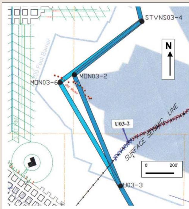
Figure 6. Measured ISS reflections points (red) were plotted on the mine map. The six reflection points shown outside of the old mine works indicate that the straight ray approach was inadequate and would require a migration solution to yield better results. As a result, the reflection points should be shifted or rotated slightly (clockwise) towards the southeast direction by about 120 to 140 ft.
