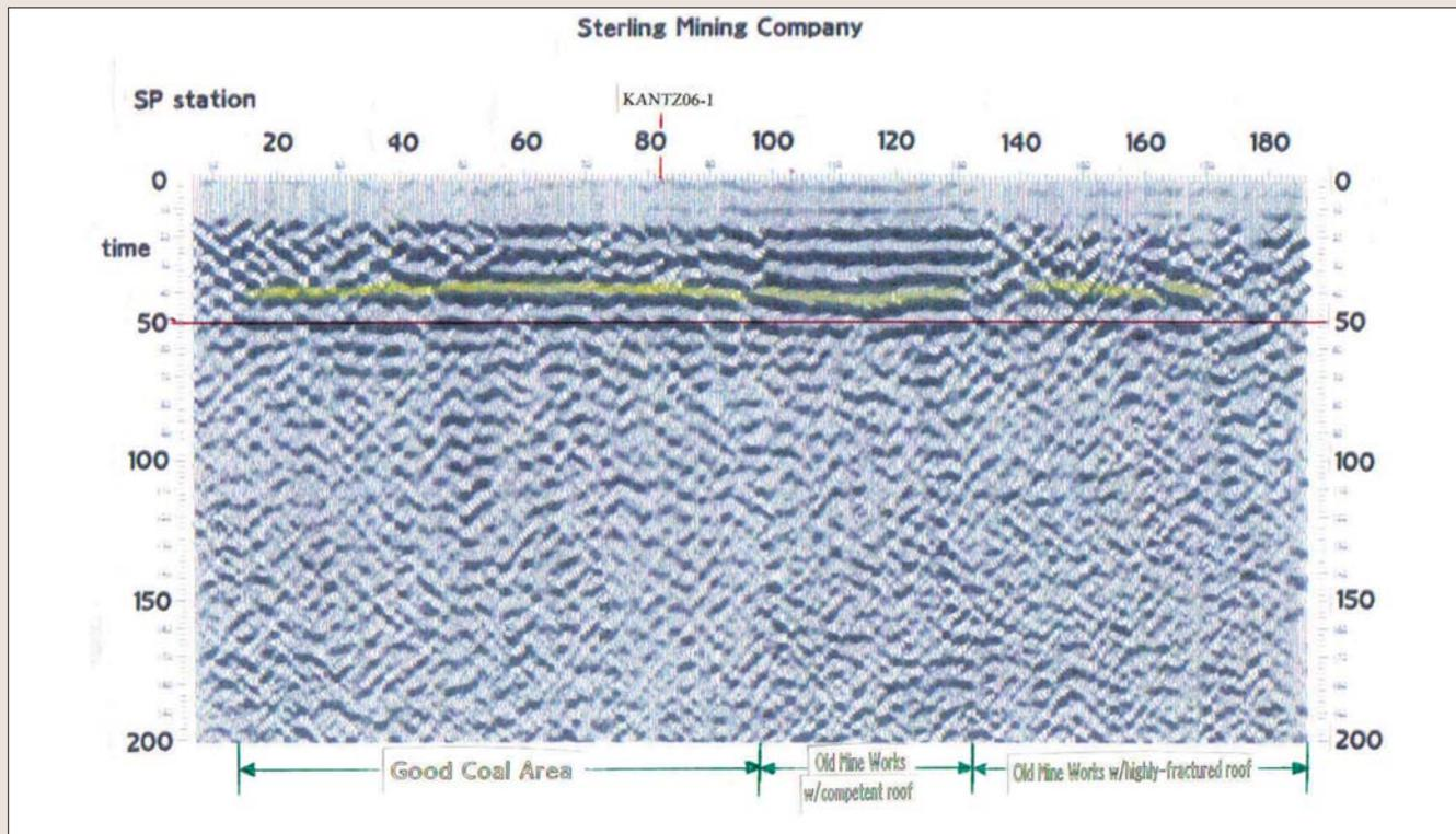
Figure 7. Interpreted seismic section of Line 3A.
