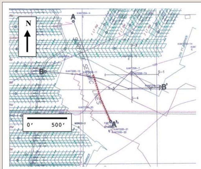
**Figure 9.** The interpreted disturbed zone beneath seismic Line 3A is shown as a red cross-hatched segment along the survey line. No disturbances associated with old mine works was detected beneath Seismic Line B.
