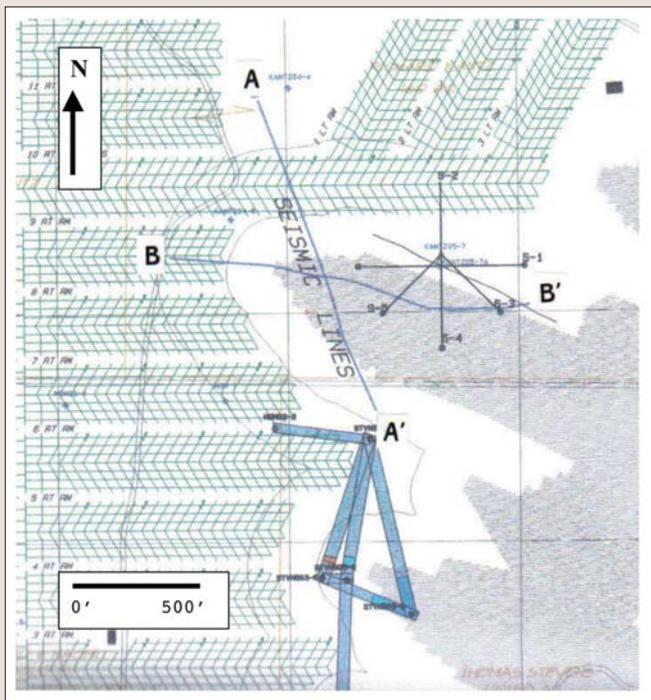
Figure 2. Expanded scale of study area showing the surface seismic Lines 2B and 3A with respect to the old Sterling Mine works (on the right). The blue-shaded arrowheadlike diagram is associated with hole-to-hole tomography surveys conducted by the coal company. Placement of the seismic survey lines was based on the concurrent understanding and interpretations of projected mine works.
