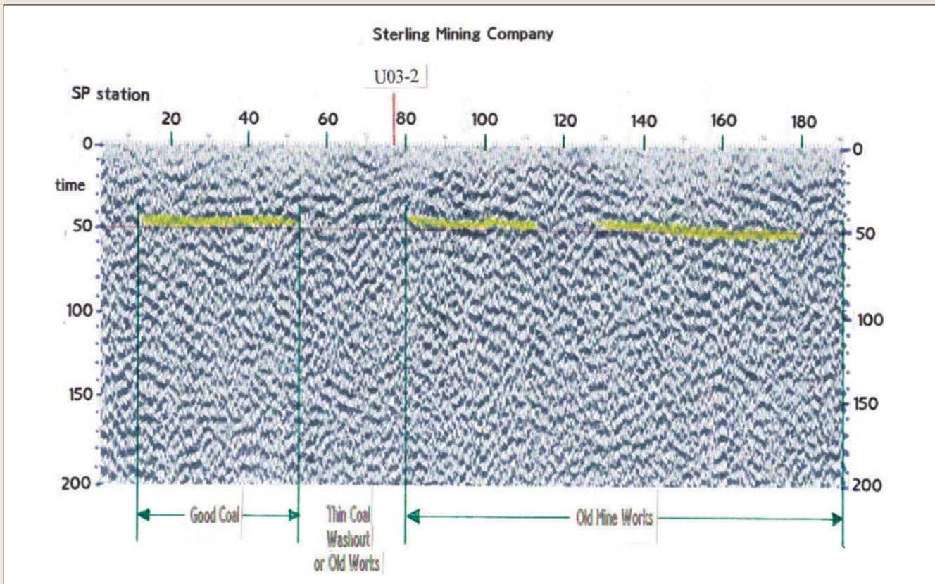
Figure 5. Interpreted seismic section of Line 1C. Borehole U03-2 near SP-77 encountered old mine works.
