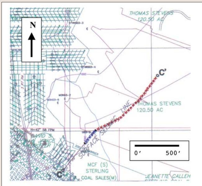
**Figure 8.** Interpreted seismic data of Line 1C is transposed on the mine map. The blue cross-hatched segment of the seismic line indicates a potential washout or old mine works. The red cross-hatched segment is associated with the old mine works.
