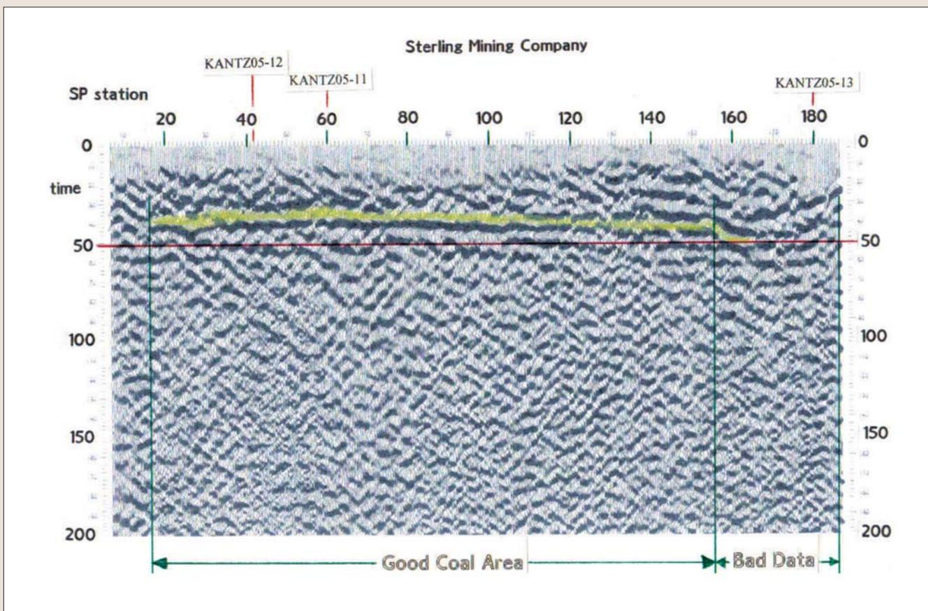
Figure 6. Interpreted seismic section of Line 2B. Vertical scale in time is ms and horizontal SP interval is 8 ft.
