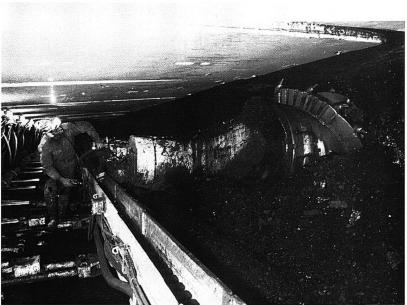
Figure 1. Miner operates the longwall where the shearer cuts the coal while the shields support the roof.
