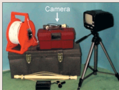
Figure 1. System components of a portable B/W, 1.25-inch diameter camera.
