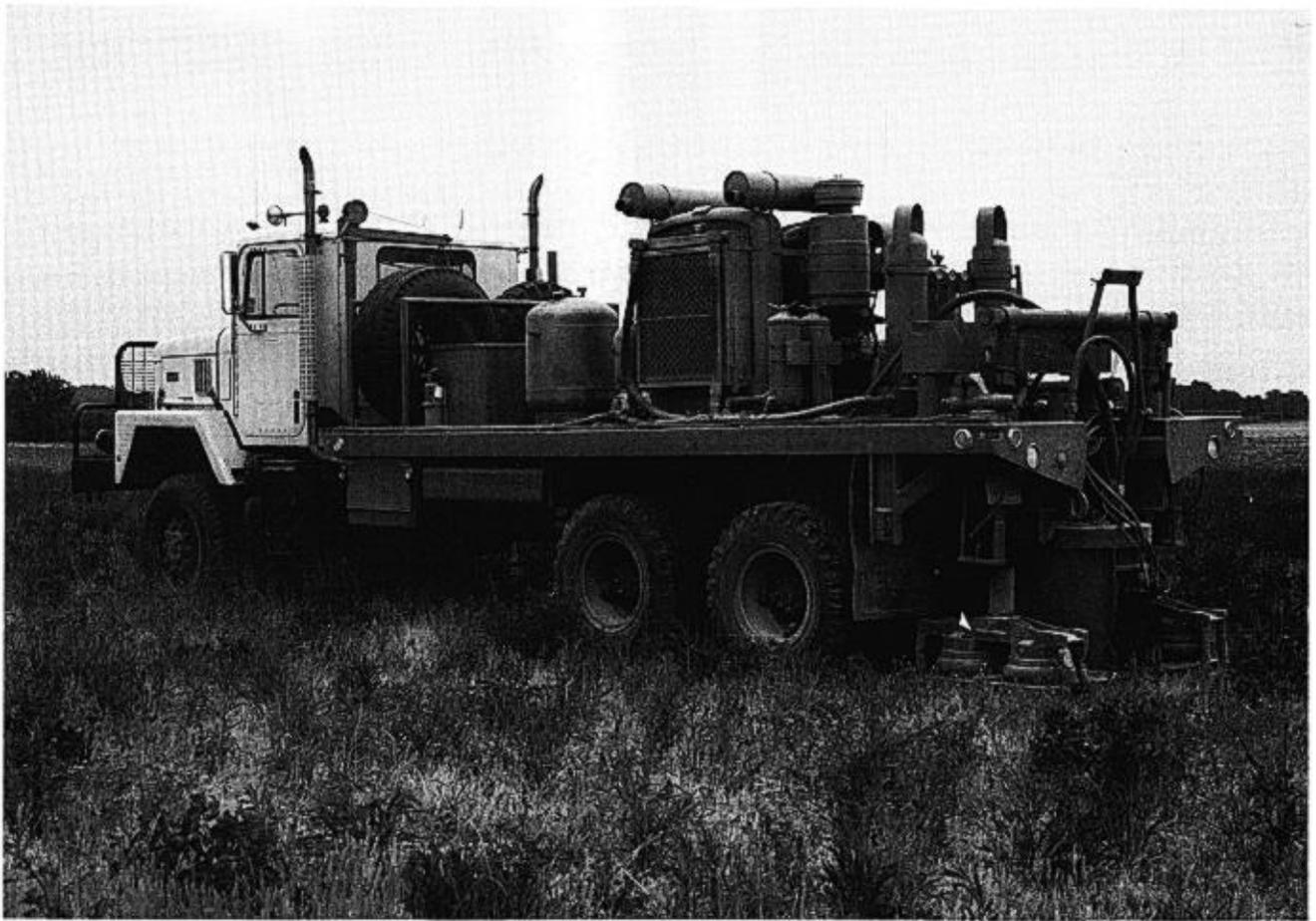
Conoco prototype vibrator being used as a high-frequency source in coal exploration.
