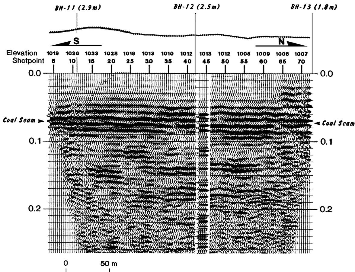
FIG. 7. The VSP seismogram is correlated to the CDP seismic section at the BH-12 location.
