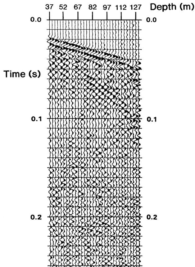
FIG. 4. VSP data after bandpass filter and automatic gain control were applied.
