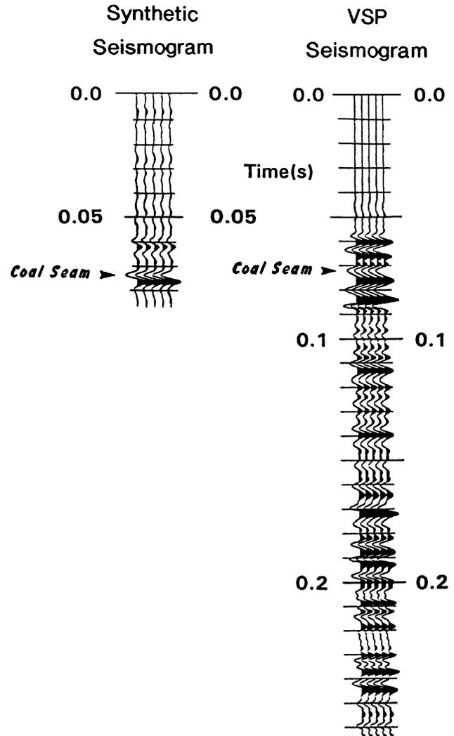
FIG. 6. Comparison of synthetic seismogram and VSP seismogram.
