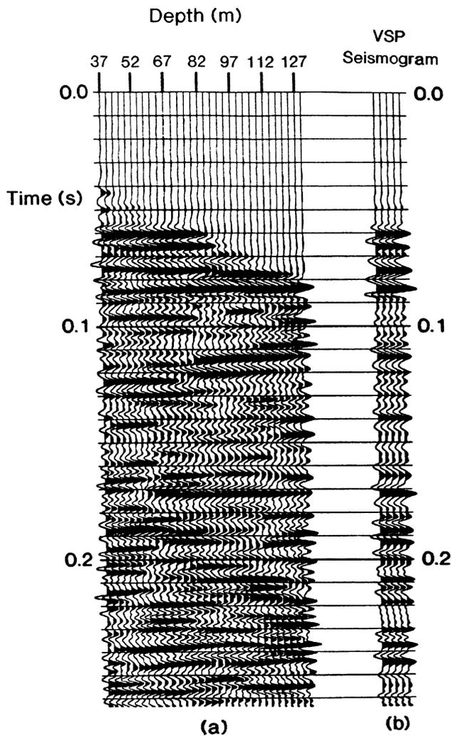
FIG. 5. Processed VSP data (a) and resultant VSP seismogram (b).
