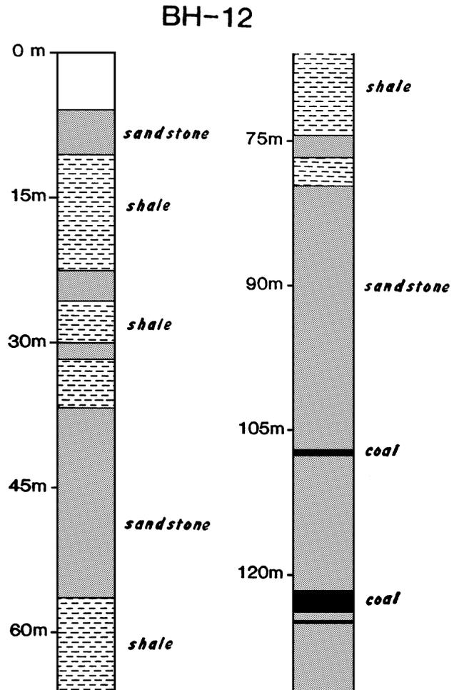
FIG. 2. Lithologic cross-section of borehole 12.
