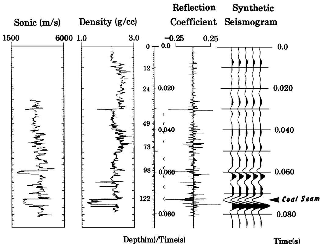
FIG. 3. Synthetic seismogram generated from sonic and density logs.
