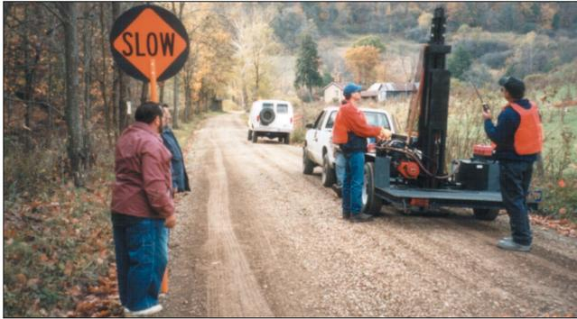
**Figure 4. High-resolution surface seismic surveying in a northern Appalachian coal field.**
